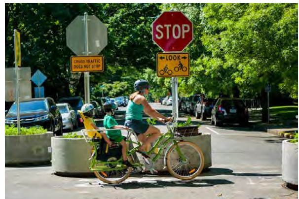
Planters can be used to divert traffic on neighborhood streets but allow bicyclists and pedestrians to pass through.
